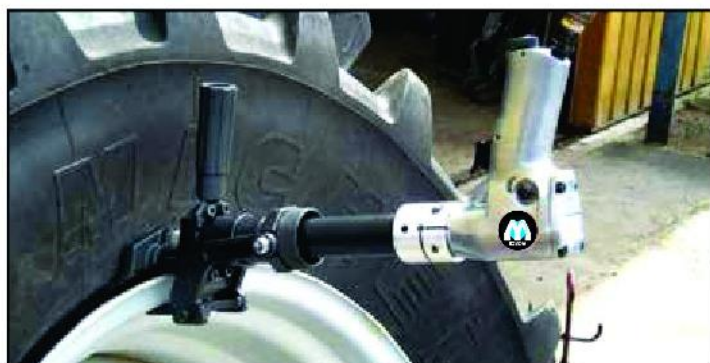
► Operation of Bead Breaker
